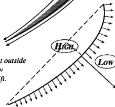
*Fig. 6 - The forces of lift include a large, unwanted heeling force and a small forward force.*
