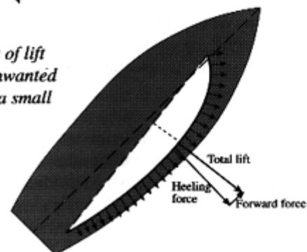
Fig. 7a - Air approaching the sail plan splits, putting the jib in a relative lift, and the main in a relative header.
