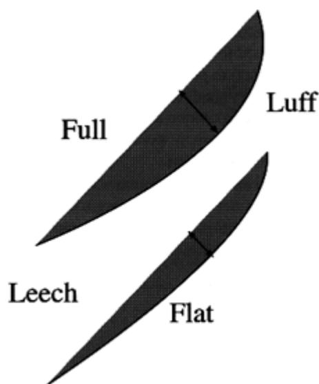
Airliners create a deep shape with the flaps down for extra lift at low speeds during takeoff and landing; but pull the flaps in for a flatter shape and less drag for high speed cruising.
