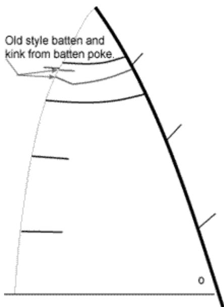
Full battens also provide a more stable platform for main sails and reduce wear from luffing and flogging. Since fully battened sails do not flog the life of a racing main will be extended enough to cover the cost of a proper set of tapered full length battens.
