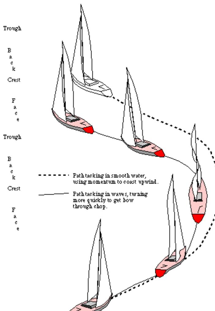
*Fig. 2 - Tacking in waves requires a faster turn than a smooth water tack. Start your turn in the trough of a wave so the bow will pop free at the crest. Try to push the bow around quickly enough so that the next wave pushes your bow toward the new tack, not back to the old one.*
