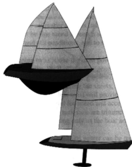
Development of higher, narrower sails is limited by sail material strength, rig engineering constraints, rules, and righting moment (heeling forces).
