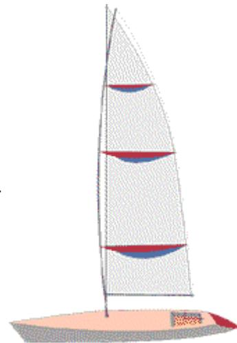
*Fig. 9 - Mast bend controls mainsail depth, particularly in the middle and upper portions of the sail. Increasing bend flattens the sail.*
