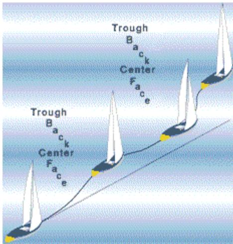
Weather helm can be used to head the boat up for each face. Rather than force the boat up with the helm the boat should be trimmed with enough weather helm that it heads itself up for each wave. In order to bear off the weather helm will have to be relieved for a moment by lowering the traveler or easing the sheet. To head up pull the traveler up, or trim the sheet. Steering with the sails and using the natural weather helm of the boat is much faster than pushing the boat around with the rudder.
