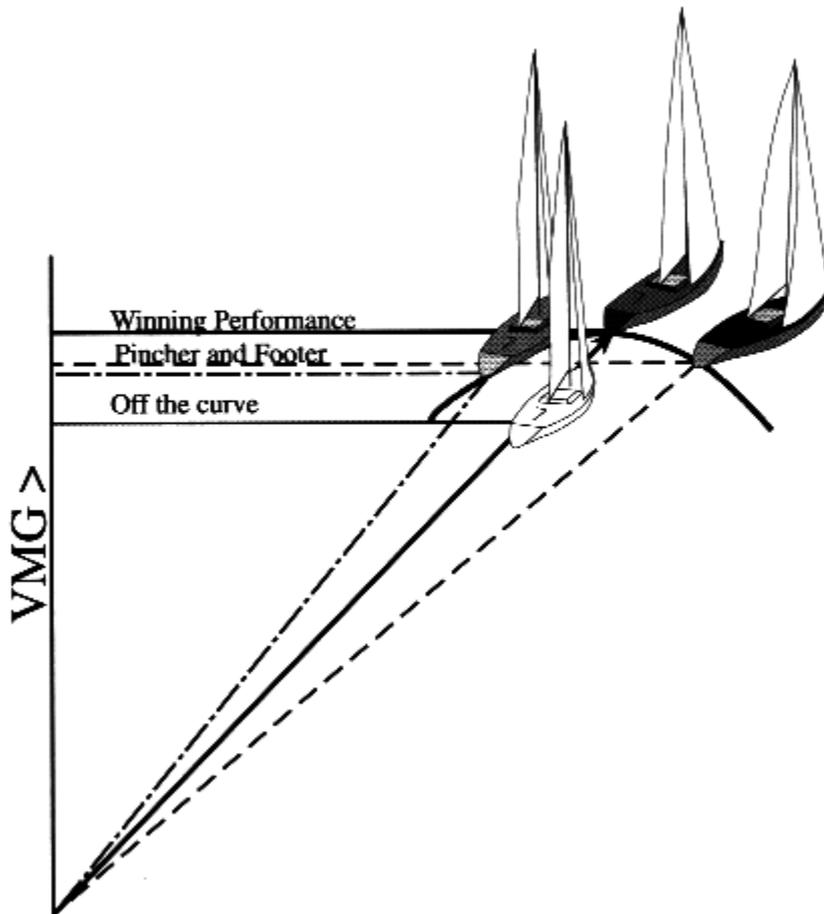
For upwind racing the goal is to achieve the optimum mix of boat speed and pointing. The figure shows a performance curve. The high point on the curve shows the best mix of speed and pointing. The boat sailing there is achieving optimum VMG - Velocity Made Good. Fig. 18.
