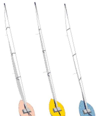
speed. The sheet should be eased to twist out the upper leech of the main when the boat is slow. Fig. 8, Boat B.
