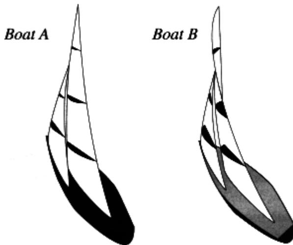
The stronger winds aloft necessitate some twist. The stronger wind up high creates a more open apparent wind angle aloft. The upper part of the sail is twisted out relative to the lower part of the sail to match the more open apparent wind angle. The sailmaker designs twist into the sail.
