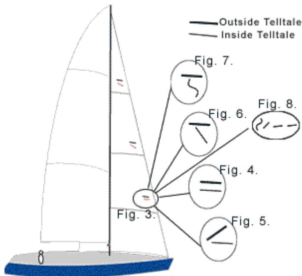
*Fig. 3 - Once you are sailing in the groove with the telltales flowing you can fine tune as follows:*
