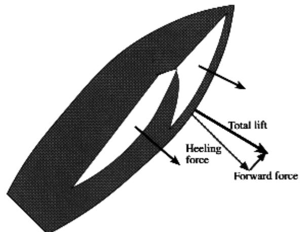
Were it not for the boats underbody, particularly the keel (or other foil), the side force would be dominant; and we would not be able to sail upwind. Fortunately, the keel generates lift which nearly offsets the side force of the sails and allows us to sail to weather (with only a few degrees of leeway).
