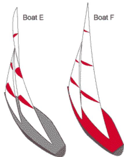
Initially the sheet's primary impact is angle of attack, pulling the boom in. As the sail nears full trim the sheet increasingly pulls the boom down (not in). At this point the primary impact of trim is a change in twist.
