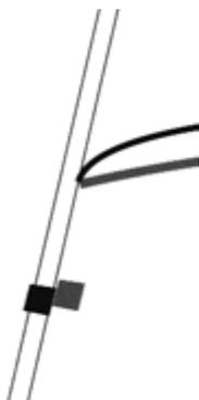
*Fig. 10 Use marks on the sail and foil to set halyard tension.*
