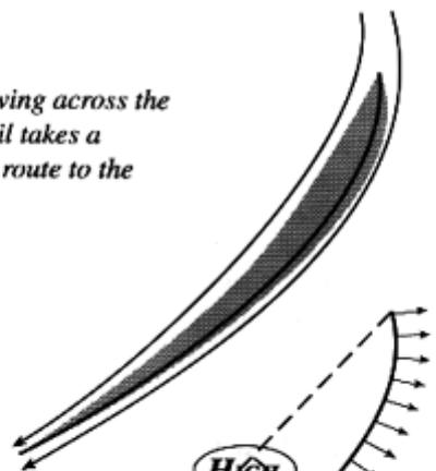
*Fig. 5 - The fast outside flow creates low pressure, and lift.*
