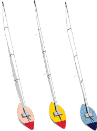
Our goal in mainsail trim is to extract the appropriate power from the main - in balance with the jib. We also seek the optimum mix of power from the three sources of sail power - angle of attack, shape, and twist. With impact on all three facets, the mainsheet is the primary control of overall mainsail power. Fig 15.
