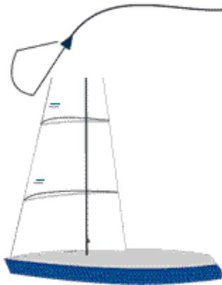
If the steering groove is wide and the boat is not pointing well try a flatter entry shape and narrower slot. Trim the sheet, tighten the headstay, and/or ease the halyard. In smooth water you will be able to steer to a narrower groove than in wavy conditions. Fig. 10.
