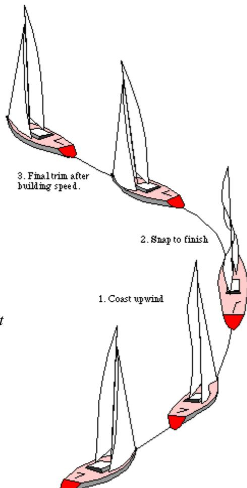
*Fig. 1 - Tacking You should always be ready to tack. The winch should be pre-loaded with a full set of wraps. The working sheet should be flaked and ready to release. Start with a smooth easy turn. Let the boat coast upwind. Release when the sail luffs half way across the deck. By grinding full speed throughout the tack overrides can be avoided and there will be no need to pause*
