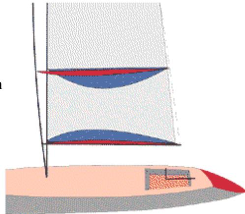
Fig. 10 - Use the outhaul to control shape in the lower portion of the main.
