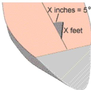
Weather helm is a key trim guide. If you are carrying more than 4° of helm, the boat is out of balance. (Note: On tiller boats 5° of helm is about 1" of helm per foot of tiller length. i.e. For a four foot tiller four inches of helm equals 5°. On wheel boats you will have to measure the ratio of wheel rotation and rudder turn.) Fig. 2.
