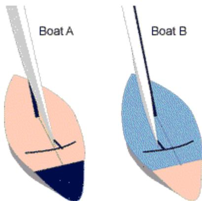
The traveler positions the boom, controlling angle of attack. Keep the boom centered (traveler to windward) until overpowered. Fig. 11.
